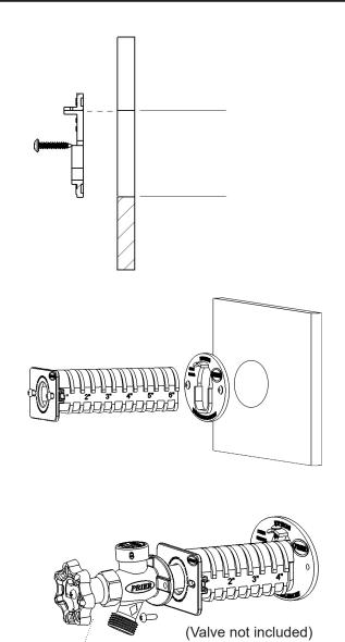
The Brick Buddy will help with the installation of most hydrants through masonry walls, however, it is designed to work best with PRIER Products, Inc. brand hydrants.
