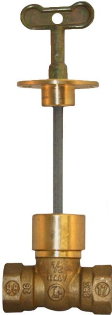
The C-67 AGA (American Gas Association) Gas Valve is for use on any gas fireplace or appliance. Using the included operating rod, the installer can install the valve from 1" to 14" depth, allowing it to be installed "below-the-joint," eliminating fittings and installation time. The C-67 Gas Valve is also used as a shutoff for any gas burning appliance.
