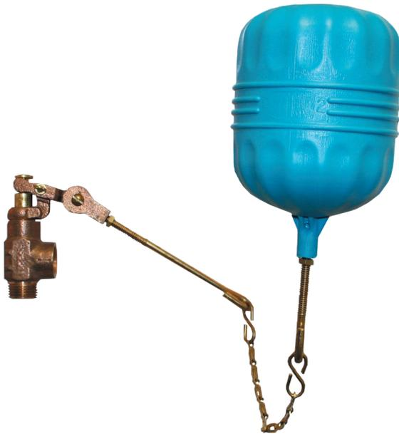
PRIER's 370 Liquid Level Control Valve is designed for cooling towers, stock tanks, poultry troughs, oil level control or any use where liquid level control is desired. The valve is heavy patterned casted brass with a neoprene valve seat. It features positive opening or closing with no leaks or chatter. The 370 Liquid Level Control Valve is available in 1/2" or 3/4" inlets. Each valve is individually tested to assure proper functionality.
