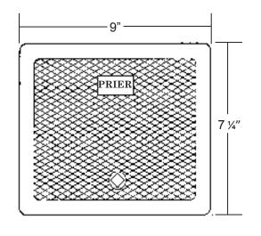
Furnish and install Freezeless Model C-734 (or C-754 with Anti-Siphon Vacuum Breaker and Backflow Check Valve) Commercial Hot & Cold Mixing Hydrant by PRIER. Hydrant shaft shall be brass with threaded and sealed connections. Hydrant shall have 3/4" hose connection with freezeless water flow and self-draining functions with brass operating rod. Hydrant shall be approved under ASSE standards. Two operating keys to be furnished with each hydrant. Hydrant insertion length to be <u>\*</u> inches.
