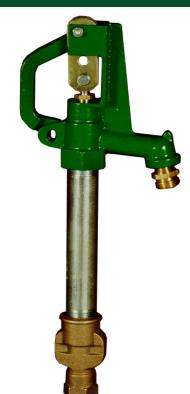
PRIER's C-240 Freezeless Ground Hydrant provides a year round source of water to areas subject to freezing temperatures. The hydrant valve is connected to the supply piping below the frost line, and since it drains automatically, it is not subject to freezing.
