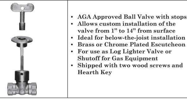
The C-67 AGA Gas Valve is for use on any gas fireplace. Using the included operating rod, the installer can install the valve from 1" to 14" depth, allowing it to be installed "below-the-joist," eliminating fittings and installation time. The C-67 Gas Valve is also used as a shutoff for any gas burning appliance.
