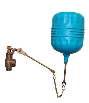
PRIER's 370 Liquid Level Control Valve is designed for cooling towers, stock tanks, poultry troughs, oil level control or any use where liquid level control is desired. The valve is heavy patterned casted brass with a neoprene valve seat. It features positive opening or closing with no leaks or chatter. The 370 Liquid Level Control Valve is available in 1/2" or 3/4" inlets. Each valve is individually tested to assure proper functionality.
